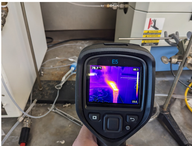
Figure 2. Thermal imaging showing the Bunsen burner flame operating in the fume hood. The horizontal stainless-steel tube above the thermal imager is the sampling line.
