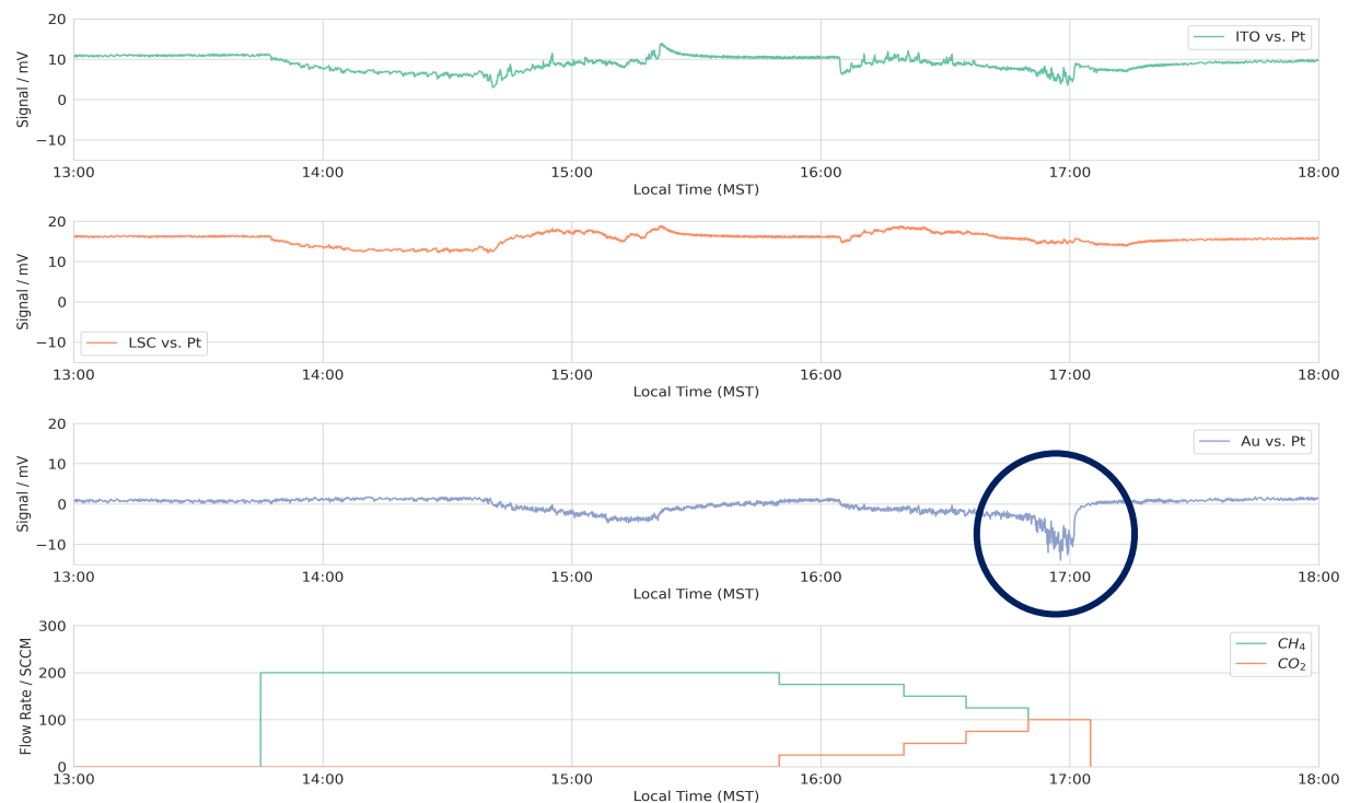
Figure 5. The simulated flameout condition was reported near 17:00. The Au vs. Pt has the most prominent early-warning and provides approximately 5 min autonomous early-warning.
